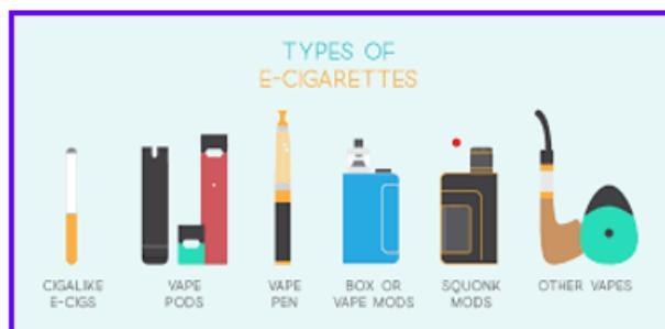
E-cigarettes are battery-powered devices that heat a liquid (usually containing nicotine, flavourings, and other additives) into an aerosol that users inhale. They **do not** burn tobacco and therefore do not produce tar or carbon monoxide, two of the most harmful elements of cigarette smoke. Most devices contain: a battery, coil (heating element), tank or pod holding e-liquid, a mouthpiece. When activated, the device warms the liquid to create vapour, delivering nicotine without combustion.
